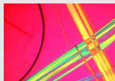
Amosite - brown asbestos during analysis
