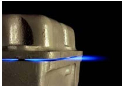
The concept is simple: put the electrical equipment to be protected in a strong enclosure that is capable of withstanding an internal explosion without bursting or without allowing the escaping hot gasses to ignite an external explosive atmosphere.
